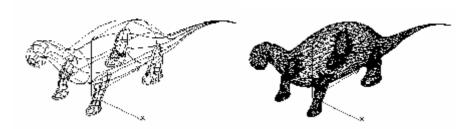
A parameter box appears requesting a *tolerance* for the faceting. This determines the *maximum distance* of the facets from the actual surface(s).
