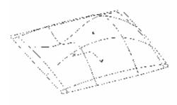
The B-spline surface is able to assume a variety of shapes that do not appear to resemble the rectangular patch structure at all. For instance, a sphere may be made and the 'rectangular' patches become like lines of longitude and latitude.
