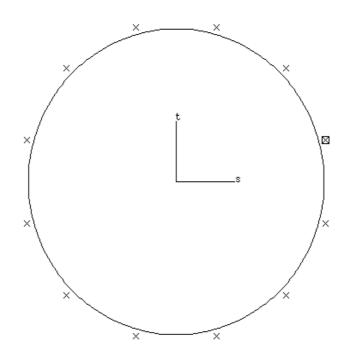
You will want to ensure that the section is *symmetrical* about the horizontal center line - there are some useful functions in curve editing to help you to achieve this. Therefore, first edit just the upper half of the curve into the desired shape.
