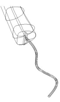
The techniques described above should be quite familiar to you. The new thing is the ability to use a single projection curve. You can have single projection curves which describe the shape of the center line of the surface, not the silhouette. In this case the size of the section curve *is* important as it determines the size of the surface. You can mix single/double primary and secondary projection sets. You could even use varying sections with a single projections.
