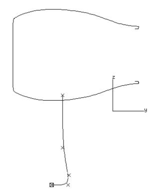
For building a surface, two projection curves are normally required. An easy way to create the other curve is to *copy* the right hand curve we have already drawn, and *mirror* it to form the left hand side of the handle.
