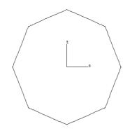
If you now re-make the surface (SURFACE $\Rightarrow$  Design: Rotate) DeskArtes will use the octagon as the cross-section shape instead of the default circle.
