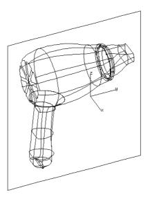
5. Issue the command TRIM⇒ Intersect: Slice, and accept the joining accuracy parameter. The command intersects all the surfaces on display with the target object (the plane).
