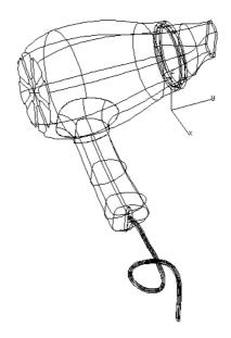
So that's to give you a taste of it. Further, it would also be possible to build a surface by scaling a section between *two 3D projections*, or even different sections if you like. But you may agree that the 2D projection curves are much nicer to interact with, and they should be used whenever possible.
