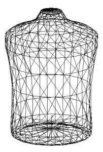
3. Wait a while and the faceted model is displayed. Finally calculate the volume enclosed by the model with DIMENS⇒ Faceted: Volume.
