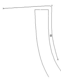
The most usual way to modify the curve is by moving the control points. Try it to make the cap follow closer the bottle neck's shape.
