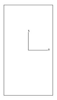
4. Enter curve edit mode [o]. Execute the global function **R**, which replaces all sharp corners with circular rounding. Accept the radius parameter value 10.
