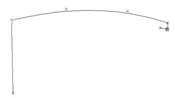
Align the left and right hand end curve parts with **1** to form right angled corners.
