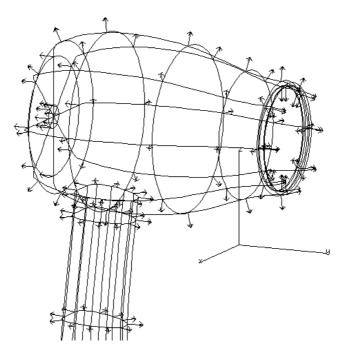
In the above figure the normals point in the "natural" directions, what you would normally consider as the outsides of the surfaces. You would then tell the system to roll the ball on the normal directions on both surfaces.
