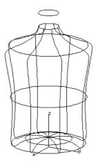
To compute the volume, the surfaces must share a consistent *normal direction*, and be changed into a *faceted model*.
