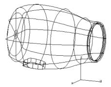
You are asked if which parts of the surfaces you want to keep. If the wrong part of either surface is displayed you must *invert* it. In the example, this (the handle) surface had to be inverted.
