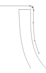
Finally let's replace the smooth corner with a numerically defined *rounding*.
