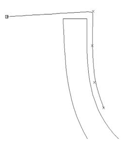
The curve's left end should be located on the vertical axis – otherwise the rotated surface will end up with a hole at the top!
