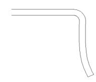
Notice that as the curves were joined, the end points became triple (sharp). Call CURVE $\Rightarrow$  Change: Edit [o] and make the triple points smoother using the **d** function.
