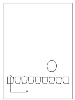
What you are seeing is the *parameter plane* of the surface. The easiest way to think of this is to image the surface to which the trim curves belong flattened out to form a rectangle. The perimeter of this rectangle is formed by the first curve in the trim curve set.
