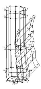
5. DESKARTES displays the intersection line. This should be a continuous loop around the finger.
