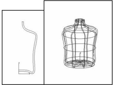
The curve only shows half of the bottle because you will finally rotate the curve 360 degrees around the vertical, z axis to make a circular bottle.
