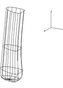
The handle appears. But – depending on the direction you drew the projection curve – the section may the wrong way around, as above. The narrow part should point ahead, not back! Read through the following even if you didn't have this problem, to know how to overcome it in the future.
